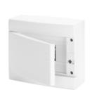
The IP40 protected decorative enclosures are available in sizes from 8 to 72M. They provide superior aesthetic integration and are equipped with screw wiring multipolar terminal blocks, 80 A IP 20. They are available with smoked transparent doors or with blank doors that can be equipped with safety lock, characterized by the "PUSH" opening and closing. The terminal blocks allow to create simple and neat wiring reducing the set-up time of the enclosure.
