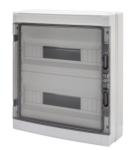
IP65 range of watertight anclosures from 8 to 72M with smoked transparent door and equipped with screw wiring multipolar terminal blocks, 80 A and IP20. The main technical features are: reversible front and back panel, removable frames and panels with windows and detechable doors with up to 180° opening and lock accessory. The terminal blocks allow to create simple and neat wiring reducing the set-up time of the enclosure.
