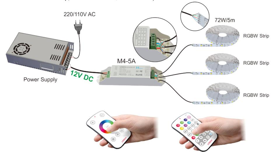
E.g. 2: Connected 24V lamp, loads 1~480W (5A×4CH×24V).
